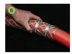
Once the cable grip is in place on the conductor, two clamps should be fitted to the end of the grip (as shown). We recommend between  $1 \frac{1}{4}$ " (30mm) and  $2 \frac{1}{4}$ " (55mm) away from the end of the cable grip.
