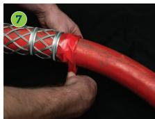
Tape should then be wound around the end of the cable grip furthest away from the eye ends.
