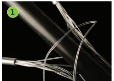
Start the lacing from the 'eye' end or anchoring end of the cable grip.
