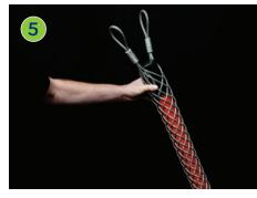
The grip then needs to be pushed along so that all the lattice is in contact with the conductor.
