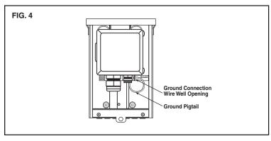
5. Install the module as follows (refer to Figs. 2, 3, and 4): Engage the module mounting clip on the left side of the rail. Press right side down until locked. Slide module down until it contacts ground block to line up LEDs with cover lenses. Connect the pigtail ground wire to a terminal on the ground block which is mounted on the rail (refer to Fig. 4).
