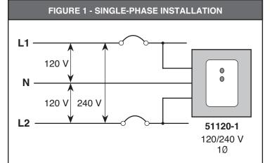
Suitable for use on a circuit capable of delivering no more than 10,000 rms symmetrical amperes, 120 volts maximum when protected by a 20 ampere circuit breaker rated 120 volts minimum. The interrupting rating of the fuse or circuit breaker shall not be less than the available fault current.
