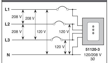
Suitable for use on a circuit capable of delivering no more than 10,000 rms symmetrical amperes, 120 volts maximum when protected by a 20 ampere circuit breaker rated 120 volts minimum. The interrupting rating of the fuse or circuit breaker shall not be less than the available fault current.
