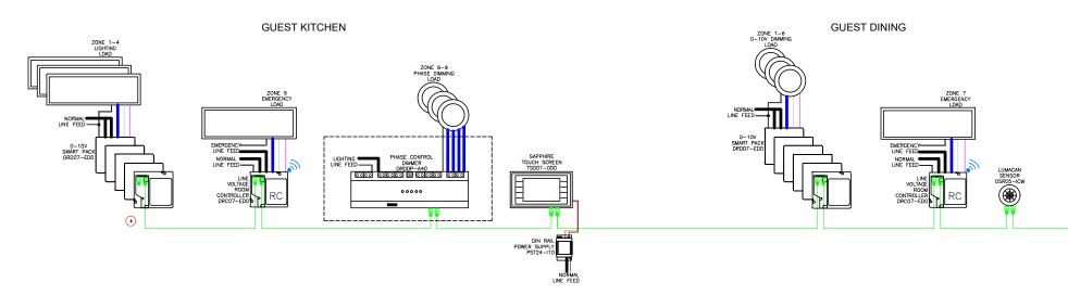
Based on Leviton GreenMAX DRC System - Leviton.com/greenmaxdrc.
