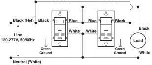
NOTE: Sensor 1 must be installed in a wall box that has both a LINE Hot and a Ground connection. Sensor 2 must be installed in a wall box that has both a Load and a Ground connection
