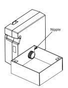
**b.** Mount to top of 4 in. sq. junction box with minimum volume 30.3 cu. in. or greater (4 in. x 4 in. x 2.125 in.) using the provided screws.
