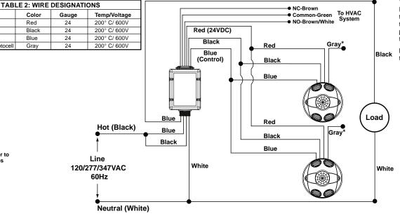
\*NOTE: When using the Photocell function, connect the Gray wire of the sensor to the Blue wire of the power pack. DO NOT use the Blue wire of sensor.
