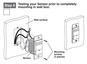
NOTE: Dress wires with a bend as shown in diagram to relieve stress when mounting device
