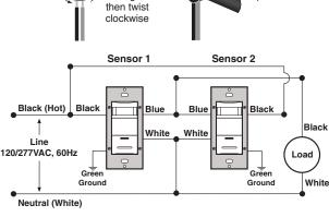
NOTE: Sensor 1 must be installed in a wall box that has both a LINE Hot and a Neutral connection. Sensor 2 must be installed in a wall box that has both a Load and a Neutral connection.
