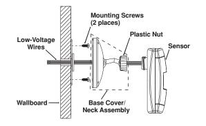
Occupancy Sensor Mounted to Wallboard or **Drop Ceiling Using Screws, Nuts and Washers**
