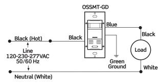
Note: Ground wire must be connected.
