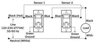
Note: Ground wire must be connected.
