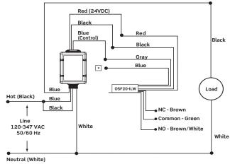
Low Voltage Wiring Diagram
