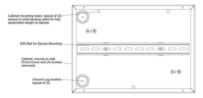
Areas marked as "(A)/(B)" are intended to be used as wire-ways. It is recommended that one side be designated for power and lighting wiring plus any other Class 1 wiring. The other side for Class 2, lower voltage wiring.
