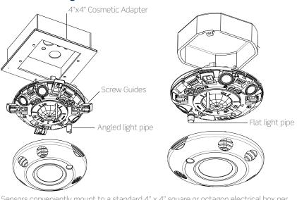
Sensors conveniently mount to a standard 4" x 4" square or octagon electrical box per NEC standards
