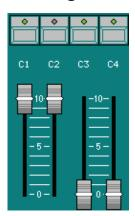
A channel can be controlled from its associated fader. The fader is used to set the channel's level by moving it to any point in its travel (from 0% to 100%). A status LED located above the fader is lit according to the level of the channel.
