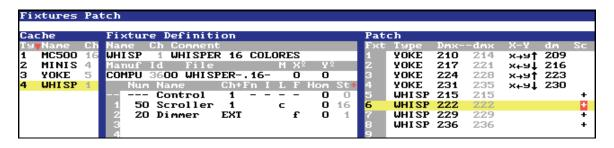
In the scroller definition table, patched scroller types can been viewed and their color names, palette assignments and gel positions (0-255) edited. In the example below, the Color5 (Step 5) gel position in Fxt 3 is being adjusted:
