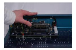
**7**. Video card should appear as shown below. **8**. Replace bottom cover. **9**. When turned on, console will auto detect monitor and video card separately.
