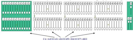
• Channel control in THEATRE/MANUAL mode. C (channel) LED's (in middle of the upper faders) are lit in green. S (submaster) LED's are lit in red:
