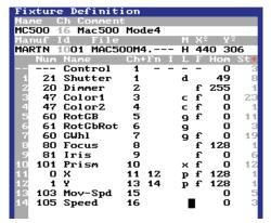
Name: Short name of fixture type. Ch: DMX channels used by the fixture. Comment: Long name of fixture type.
