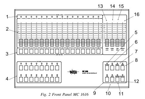
These 16 buttons are used to bring an individual channel, to full intensity. They also are used for quick pattern programming.
