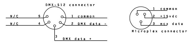
Fig. 1 Dimmer Output Connectors
