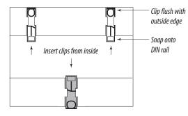
3. To reduce horizontal shifting across the DIN rail, use two end stop clips.
