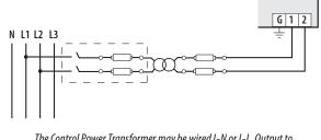
The Control Power Transformer may be wired L-N or L-L. Output to meet meter input requirements
