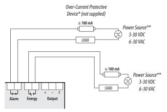
The solid state pulse outputs are rated for 30 VAC/DC nom.
