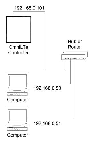
To connect to an Omni LTe controller on a local network using LEVITON PC Access, under *Configure* >> *Network* enter the controller's IP address:
