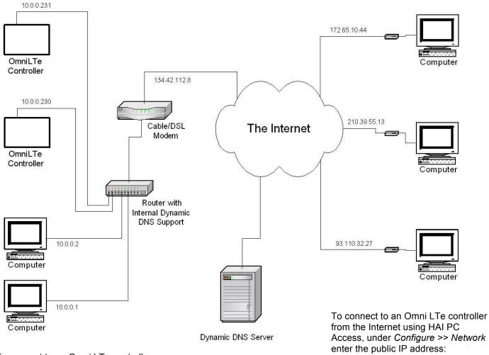
To connect to an Omni LTe controller on a local network using HAI PC Access, under *Configure >> Network* enter the controller's IP address:
