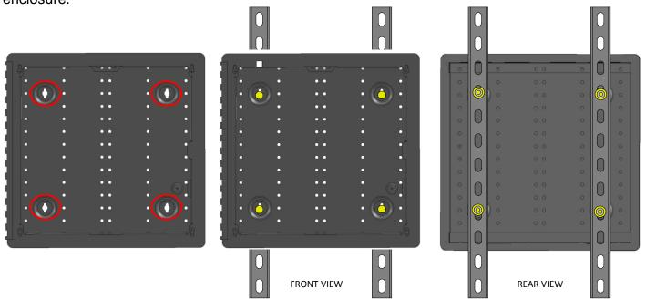
The use of steel channel is recommended to provide a mounting point for threaded rod (recommended), hanger wires or other support hardware (non-Leviton materials).
