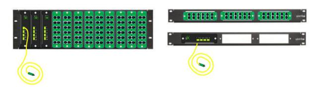
The flush mount panels can be mounted in consolidations point enclosures with a minimum of 2RU mounting spaces. Consideration should be made for rack unit rails with an angled orientation to allow for proper bend radius control and cassette depth.
