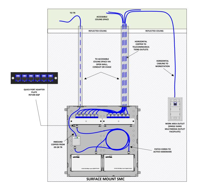
Summary – SMC Enclosures are compatible with the Opt-X PON solution and Quick Port connectors, providing flexibility and ease of installation in both ceiling and wall mounted, non-plenum environments. For more information go to: <u>www.leviton.com/OptXPON</u> and <u>www.leviton.com/SMC</u>.
