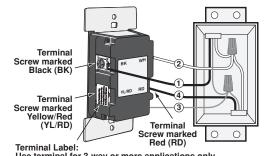
Use terminal for 3-way or more applications only. For single-pole applications, DO NOT remove label.
