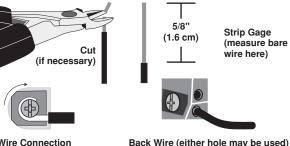
Side Wire Connection Side wire terminals accept #14 AWG solid wire copper only.
