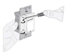
Using a flat screwdriver, push in upper and lower tabs on left side of frame, then rotate right to release face
