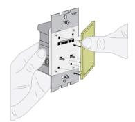
Line up and insert right side tabs, then rotate left to attach new face
