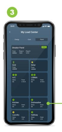
Tapping on a breaker opens a breaker details screen. From here you can view breaker info, rename it, set the position, edit notification settings, and more
