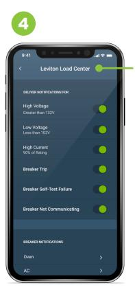
The My Leviton app provides peace-of-mind with alerts and notifications for unusual electrical activity, including when and why a circuit trips, high or low voltage events, if the breaker fails a self-test, or if communication is lost
