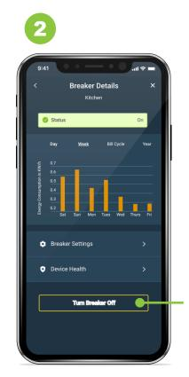
2nd Gen Smart Breakers can be turned ON or OFF remotely
