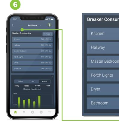
Breaker Consumption widget shows a breakdown of smart breaker consumption per circuit.
