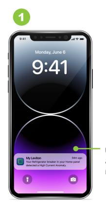
Users can select Smart Anomaly Detection to receive alerts if unusual activity is identified, such as a freezer not running, or an HVAC system running for too long
