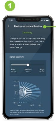
The motion calibration tool can be used to select the right sensitivity/coverage range for the environment
