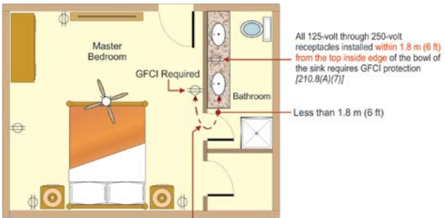
When determining if GFCI protection for personnel is required and a measurement is involved, the distance from a receptacle is required to be measured as the shortest path the supply cord of an appliance connected to the receptacle would follow without piercing a floor, wall, ceiling, or fixed barrier, or the shortest path without passing through a door, doorway, or window [210.8]
