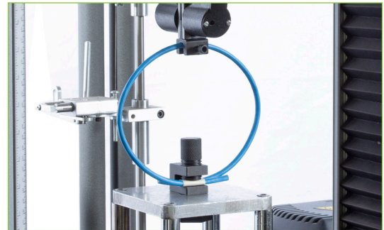
Figure 1: A highly specialized piece of equipment measures the Pound Force (LbF) exerted onto the cable sample
