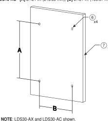
**b.** To calculate mounting screw length, add the board/wall ② thickness to the thread engagement ®. Thread engagement into enclosure @ must be between 0.5 in. and 1.0 in.
