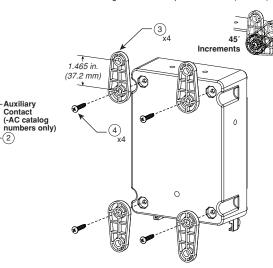
**b.** Attach mounting feet ③ with provided Plastite® #8-16 x 7/8 in. c. Mount unit to the wall using the 0.28" (7.1 mm) diameter clearance holes in the mounting feet. Mounting screws (5) not
