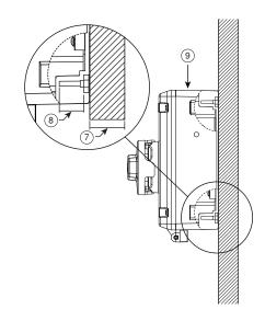
c. Mount unit to the board/wall ① with four #8-16 Plastite® thread forming screws (1) (not provided). Torque to max. of 15 in-lbs.
