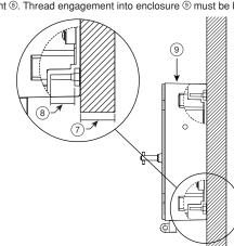
c. Mount unit to the board/wall 7 with four #8-16 thread forming screws 10 (not provided). Torque to max. of 15 in-lbs. (1.7 N-m).
