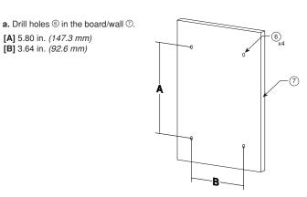
**b.** To calculate mounting screw length, add the board/wall  ${\mathbb O}$  thickness to the thread engagement ®. Thread engagement into enclosure 9 must be between 0.5 in. and
