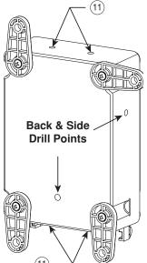
d. Mount unit to the wall using the 0.28 in. (7.1 mm) diameter clearance holes in the mounting feet. Mounting screws (5) not provided. NOTE: Verify enclosure is level prior to mounting.
