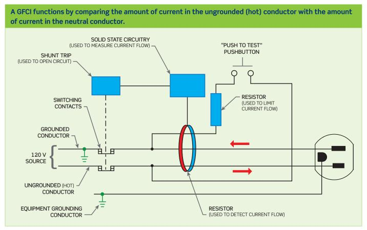
leakage current exceeds a selected level, the GFCI would open the circuit, removing the source of energy. (See Figure 7, above).
