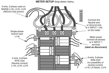
NOTE: The VerifEye meter series uses the NEUTRAL terminal as a voltage reference. For systems without a neutral conductor, Leviton suggests connecting a ground wire to this terminal. If the neutral terminal is left open, L-L measurements are accurate, but L-N measurements may not be symmetric. If a ground wire is connected to the NEUTRAL terminal, <2 mA flows into the ground wire.
