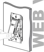
b. With the front faceplate of the sensor removed, push both buttons on front of sensor simultaneously for 10-15 seconds (note: after 5 seconds, a light will blink BLUE and then alternate between BLUE and RED) and release when the Locator Light is blinking GREEN.
