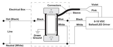
· Use this device with copper or copper clad wire only.
