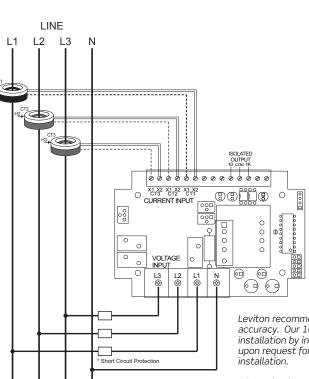
Leviton recommends solid core transformers (CTs) for revenue-grade accuracy. Our 100A and 200A color coded CTs assist with correct installation by indicating phase monitored. Split core CTs are also available upon request for applications where power cannot be interrupted during
