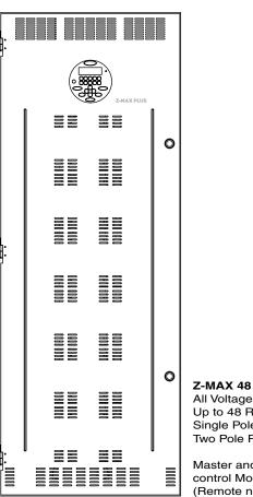
All Voltages Up to 48 Relays Single Pole and Two Pole Relays
