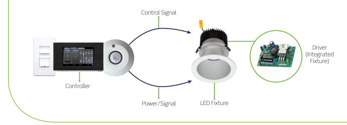
When planning an LED control solution, it is important to understand that **different driver types require different solution technologies.** In order to ensure a compatible solution, first determine:
