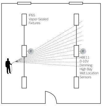
NOTE: Combine IP65 vapor-sealed fixtures (supplied by others) and Leviton HBE11 high bay wet location sensors for complete wash down application safety.
