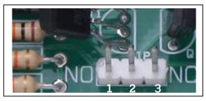
Jumper position for Last State (no pins)
