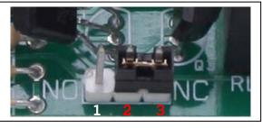
Jumper position for (NC) Normally Closed (pins 2 and 3)
