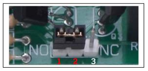
Jumper position for (NO) Normally Open (pins 1 and 2)
