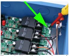
Figure 4 - Mounting Screw Removal
