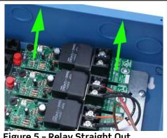
Figure 5 - Relay Straight Out
