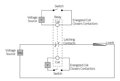
Typical Latching - Mechanically Held Relay
