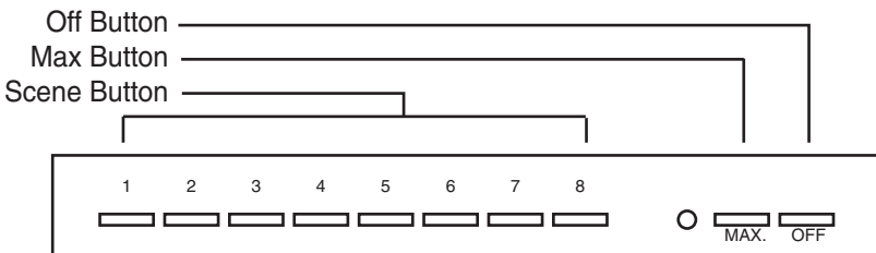
Figure 14 - Scene, MAX and OFF button Locations
