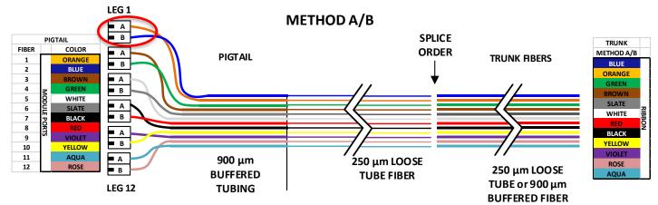
Method A/B, Option 2 – Leave the connectors in the A/A positions and fusion splice the fibers in a pair-wise flipped method.
