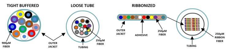
Terminating two ribbonized fibers together is typically achieved with a fusion splicer specifically designed for splicing multiple fibers. Fusion splicing of all fibers occurs concurrently. While terminating ribbonized fiber to other fiber constructions is possible, it requires additional preparatory steps, tools and equipment and is not addressed in this document.
