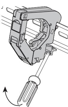
2. While pushing the sides outward, pull the loading arm forward to place the module into loading position.
