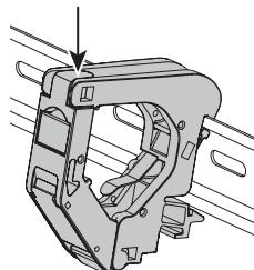
3. Load the jack to be installed by orienting the latch with the UP indicator on the module. Capture the bottom ridge of the jack and then rotate it into place. A flat blade screwdriver may be used to depress the tab as needed.
