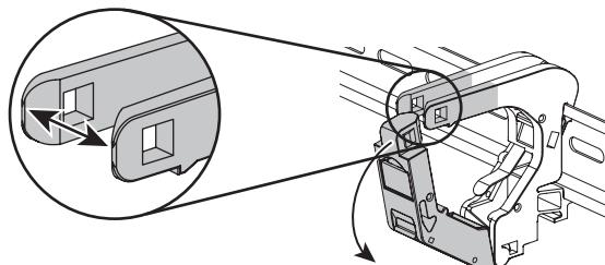
4. Guide the cable between the module sides, while closing the loading arm. Optional side covers may now be installed.
