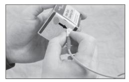
**b.** Contact the ferrule end face to the wet area and gently drag to the dry area of the wipe.
