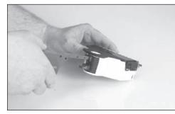
Clean all components in each mated pair before connection. This includes the connectors on all trunk assemblies, patch cords, ports of a cassette or adapter plate.
