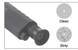
Visually inspect each mated pair. Use a 200X field microscope or video scope to verify end face cleanliness. If contamination is present, clean and re-inspect each mated pair before connection.
