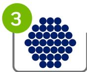
**Prevent crushing lighter weight cables by positioning Cat 6A cables on the bottom of cable trays and limit bundles to 50.** On conduits and trays, use stronger, properly sized anchors, threaded rods, and J-hooks. Space supports randomly between three and four feet apart to prevent cable bundle sagging.
