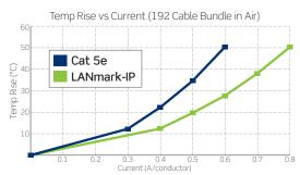
**LANmark-IP** stays 44% cooler than traditional Cat 5e cables under the strain of 100-watt PoE.
