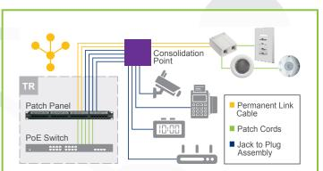
**Passive Zone** — Like home run cabling, this type of architecture locates all active gear in the telecommunications room. However, a consolidation point is added between the telecommunications room and the devices to facilitate moves, adds and changes.
