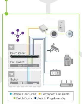
Active Zone — In this architecture, a PoE device is located in the telecommunications enclosure to accommodate long distance runs between the telecommunications room and the telecommunications enclosure, or to facilitate the transmission of large amounts of data. The cabling from the telecommunications room to the telecommunications enclosure is typically fiber, with copper cabling running from the telecommunications enclosure to the devices.
