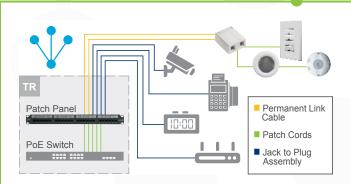
**Home Run** — In this network architecture, all active gear is located in the telecommunications room with permanent link cabling running from the telecommunications room patch panel to each device. A surface mount box or other type of termination at a port may also be included, with patch cords connecting to the devices.
