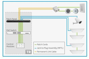
the way back to the TR. For example, if the security camera needs to be moved five feet closer, there might not be an issue, but if it moves five feet farther out, there might not be enough cable and the entire link will need to be reworked.
