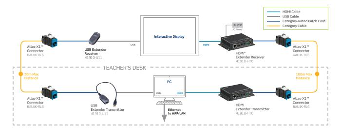
An up-to-date audiovisual network built on standards-based category-rated cable allows schools to minimize the high costs associated with complete network upgrades. Plus, since these plug-and-play solutions do not require programming, and often can be added to an existing certified permanent link, a datacom expert can quickly perform the installation, allowing a single contractor to facilitate all datacom and audiovisual networking needs.
