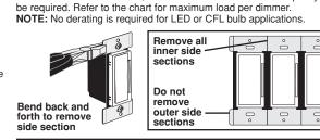
In multi-dimmer installations, the reduction of the dimmer's capacity may
